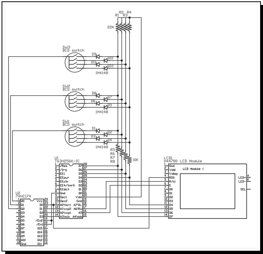
The method for reading the switches in this circuit are identical to that used for the previous circuit with the additional requirement that the LCD may alter the selection value and thus the switch selection needs to be updated before any switch is read.
