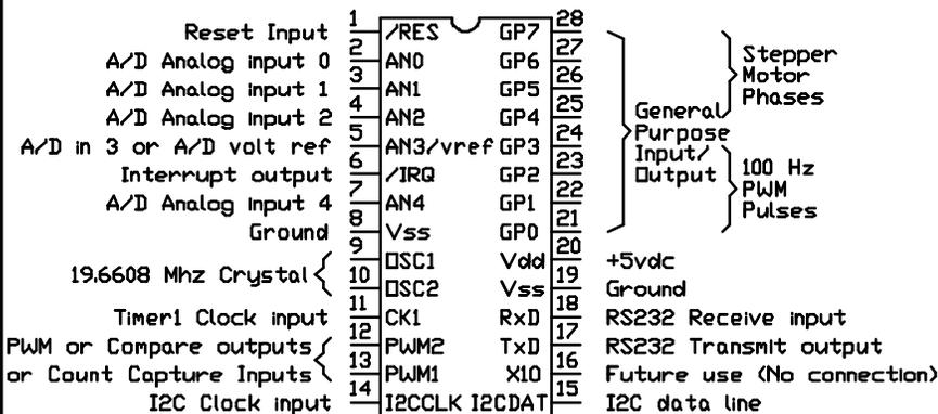
Only the I2C clock and data lines, the Reset line, Ground, and the Interrupt line are connected to the host processor. The Xtender device requires a 19.6608 Mhz Cryxtal, two 12pf capacitors, and two pull up resistors for the I2C lines. The small number of components and connections simplifies construction and layout of prototypes and the final product.
