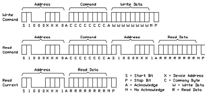
This command protocol is accomplished in FBASIC with the `i2c_write` and `i2c_read` functions. Both functions require a word parameter where the high byte is the address and the low byte is the command. The `i2c_read` function returns the byte sent from the Xtender. The `i2c_write` function sends the second parameter to the Xtender.
