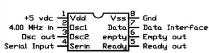
1. Vdd - +5 vdc power supply for the device
