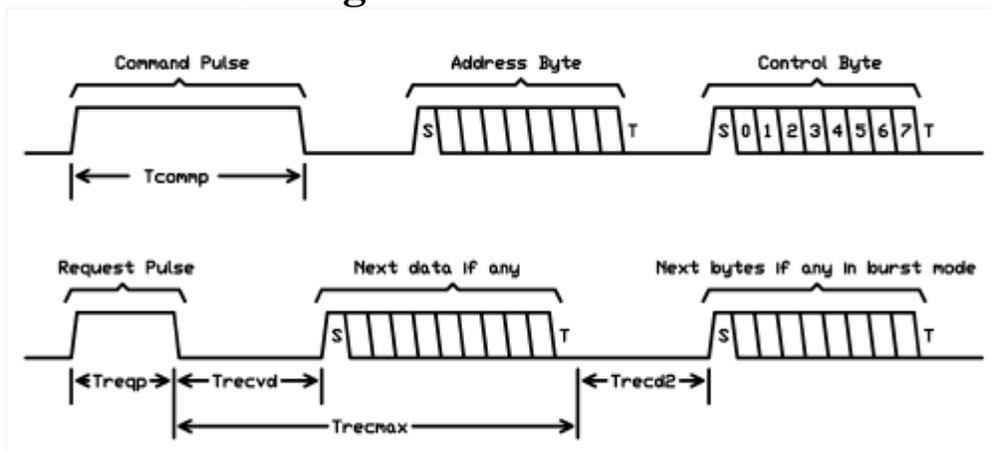
**Operational Timing Parameters:** Condition: Osc=4MHz
